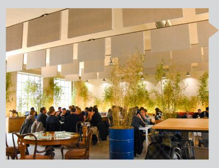
SEALED AIR® brand Whisper® Acoustic Panels were installed as vertical baffles from the ceiling, in such a way that they did not impact on the original architecture of the vault.
